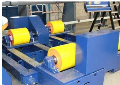
The supports can be motorised to easily move a shell along the rails.
