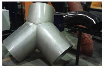
While Enerflex purchased the SPC 2500 to cut holes in pressure vessels, the company is now realizing dramatic productivity on other parts as well. The black piping (or lobster back) shown on the right used to take 10 hours to cut and fabricate. It now takes around an hour.
