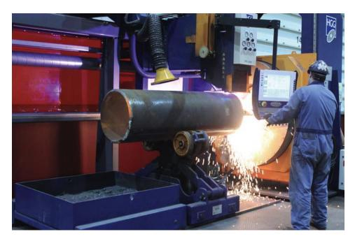
The SPC 2500 has automated and simplified the way Enerflex lays out pressure vessel hole locations and cuts the beveled holes. It used to take about 8 – 10 hours to prepare a typical shell to weld in the nozzles. Now the entire process takes about one hour.
