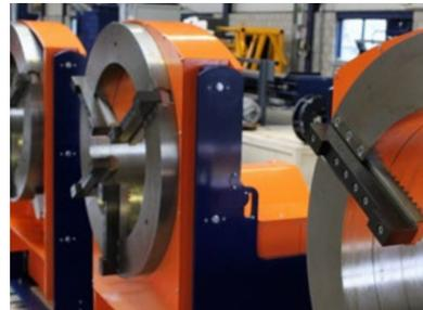
A 4-jaw chuck is used to clamp both pipes and box sections. Pipes and box sections are rotated very precise, resulting in highly accurate cuts and less grinding afterwards.
