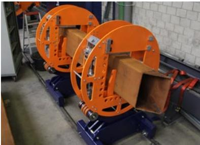
Both pipes and box sections are cut on the same supports. However, to easily rotate box sections, HGG has developed a special rotator with easy loading from the top.
