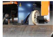
For accurate cuts, the RBPC can measure and compensate longitudinal movement of the pipe during rotation (creep) and circumference deviation of the pipe.
