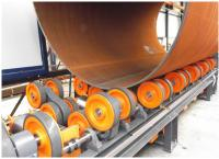
The roller bed is used to rotate and support the pipe. The tandem wheel sets can smooth unevenness of the pipe surface (like weld seams) to prevent vibrations during cutting and obtain accurate cuts.
