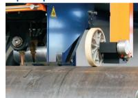
For accurate cuts, the RBPC can measure and compensate slip during rotation of the pipe.
