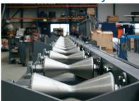
To even further improve the productivity of the RBPC, it can optionally be equipped with an in- and out-feed system. This will speed up handling time of the pipes.
