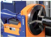
The self-centring three jaw chuck is one of the factors influencing accuracy. It achieves high accuracy by clamping pipes securely, avoiding slip and creep (longitudinal movement) during rotation.
